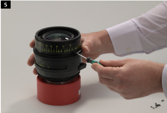
Loosen the nine screws by using the T4 Torx Screwdriver.
