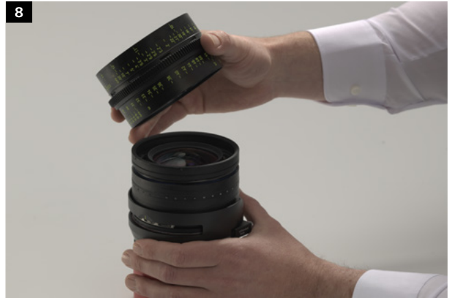
Turn the focus to the end stop and flip the scale ring around so that desired scale is on the down side.
