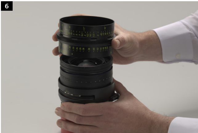
Lift the scale ring and take it off the lens.
