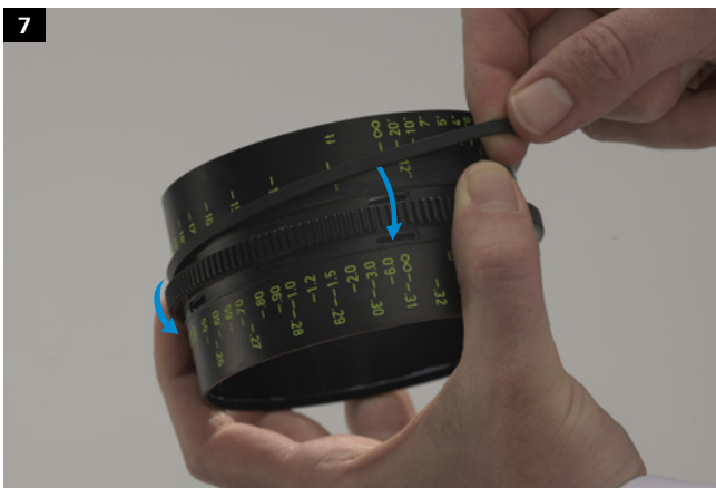
Remove the rubber ring of the scale ring, and put it on the other side of the scale ring. The rubber ring always has to be on the bottom side of the scale ring.
